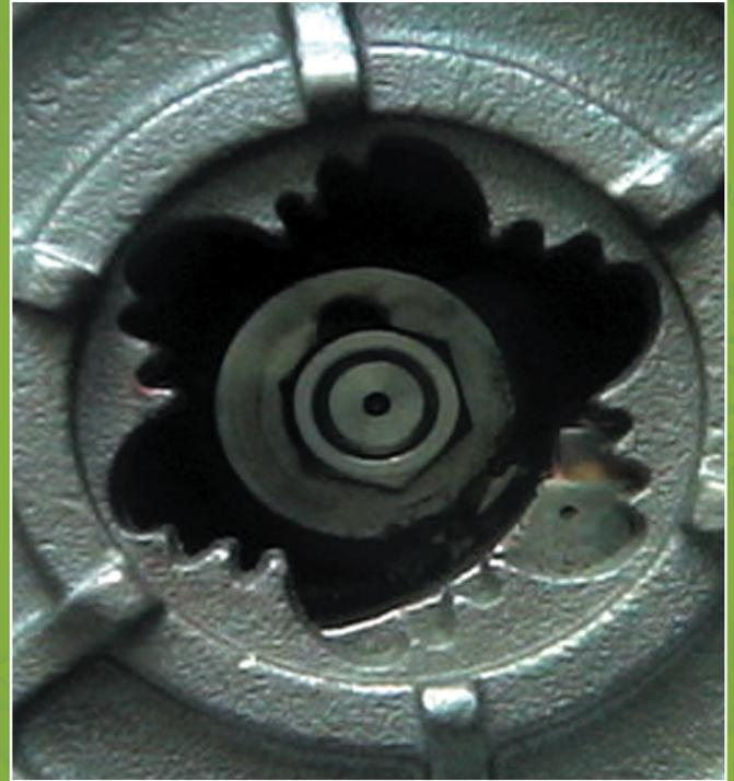
**Shredder pumps can handle most unintended items that occasionally enter the waste stream.**
